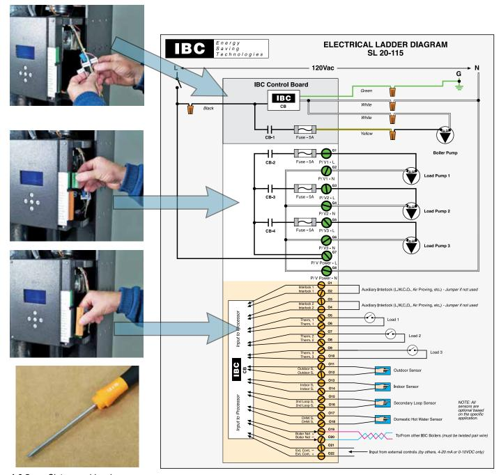
A 2.5 mm Slot screwdriver is required for the bottom terminal strip. Broader or narrower blades may damage the terminal screws.
