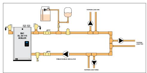
Figure 24: Basic Primary/Secondary piping with closely-spaced tees concept
