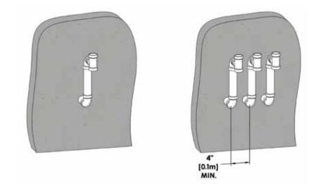
Figure 6: Sidewall vent termination - indoor combustion air applications
