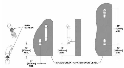
Figure 5: Sidewall vent termination - piping configuration
