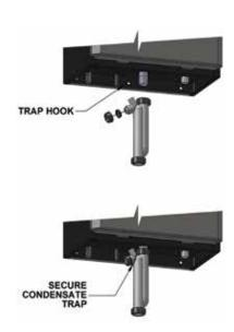
Figure 16: Condensate trap installation
