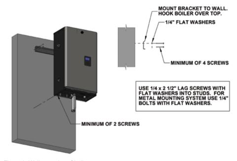
Figure 2: Wall mounting of boiler
