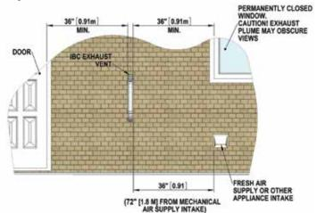
Figure 10: Vent terminal clearances
