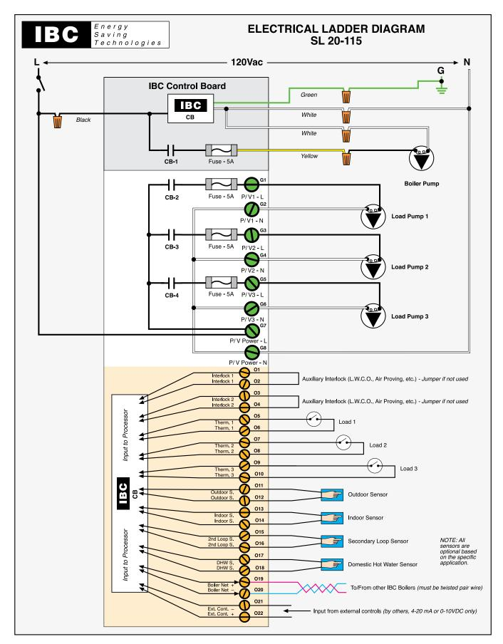
Diagram 6.2-2: Ladder wiring diagram
