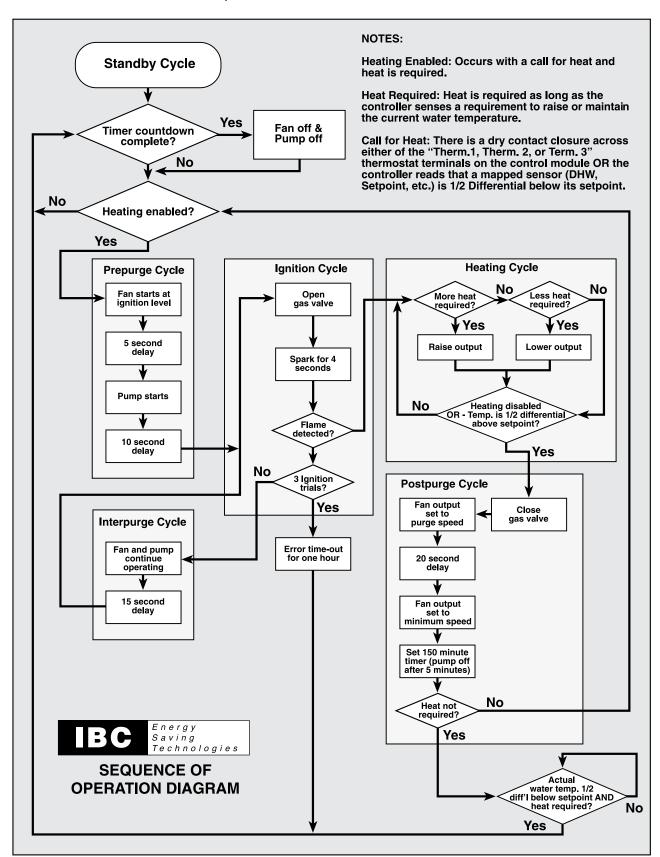
Diagram 6.3: Sequence of operation diagram
