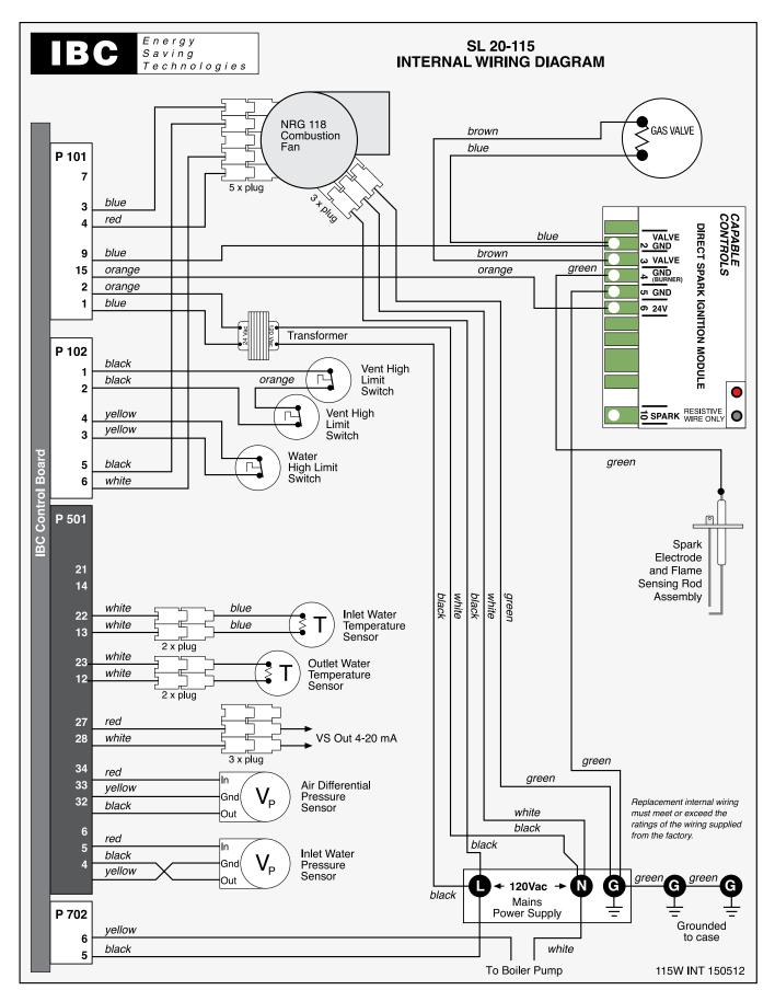
Diagram 6.2-3: Internal wiring diagram
