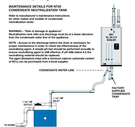
Figure 19: Condensate neutralization tank
