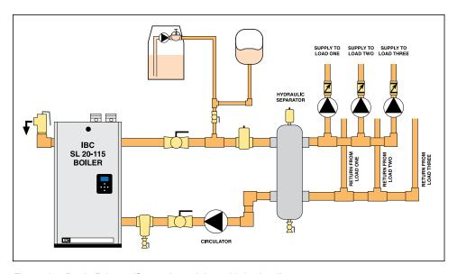
Figure 27: Basic Primary/Secondary piping with hydraulic separator concept
