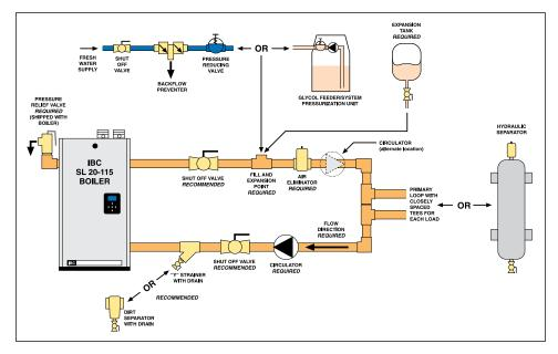
Figure 23: Boiler trim basic options - side piping
