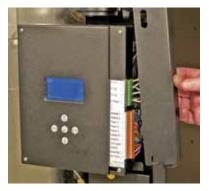
Removing circuit board terminal cover
