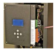
Remove terminal plugs, then circuit board cover
