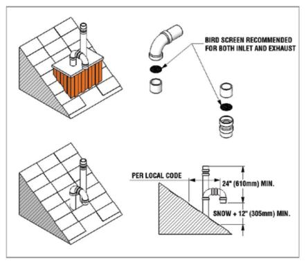
Figure 4: Rooftop vent terminal configurations
