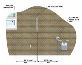
Figure 11: Vent terminal clearances
