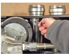
Removing vent stack test port plug
