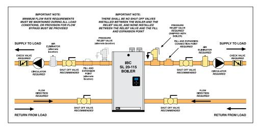
Figure 31: Parallel piping connection to two sides
