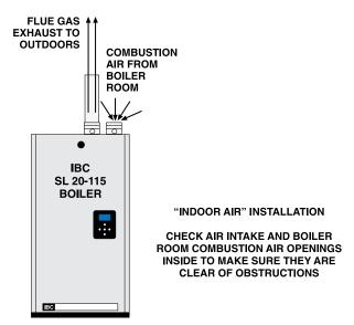
Figure 13: Indoor combustion air intake
