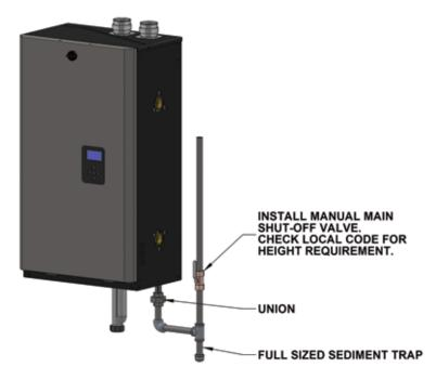
Figure 35: Typical gas piping connection
