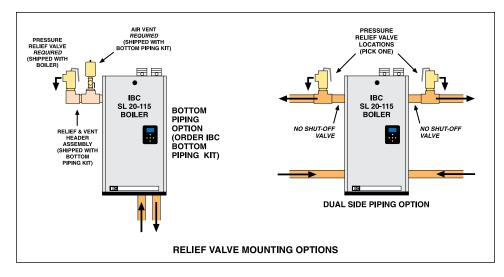
Figure 22: Relief piping with dual side or bottom piping connections
