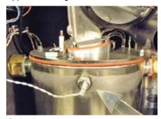
Outlet (supply) water temperature sensor
