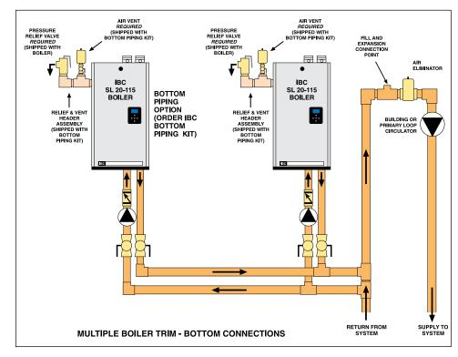
Figure 34: Multiple boiler piping concept
