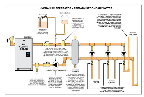
Figure 28: Important Primary/Secondary piping details with hydraulic separator
