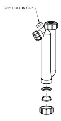
Figure 17: Condensate trap disassembly for cleaning
