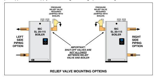
Figure 21: Relief piping with single side piping connections
