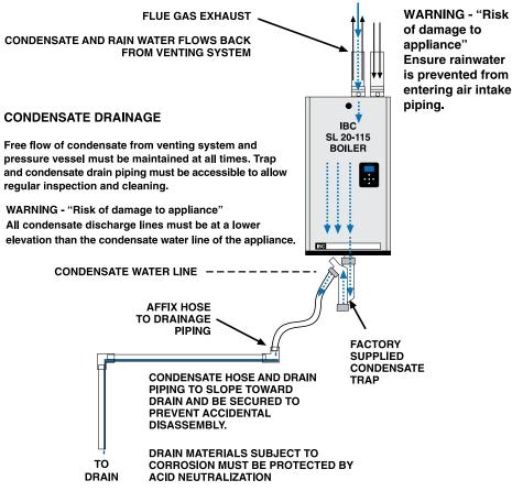
Figure 18: Condensate trap drainage
