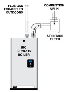
"DIRECT VENT" INSTALLATION WITH INTAKE AIR FILTER
