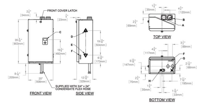
Figure 1a: Dimensions / Connections for SL 20-115
