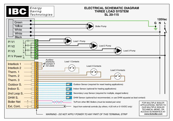
Diagram 6.2-1: Pictorial wiring diagram
