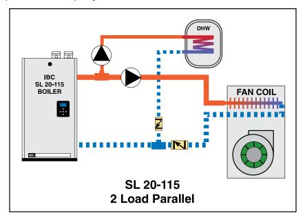
Figure 33: Two pump, two load - parallel piping concept
