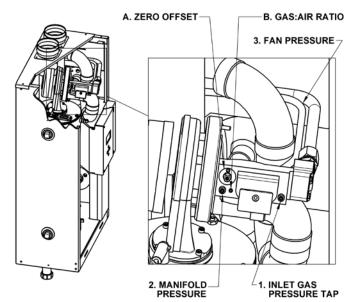
Figure 38: Gas Valve and Pressure Reference System
