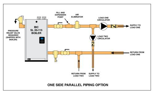
Figure 30: Parallel piping connection to one side
