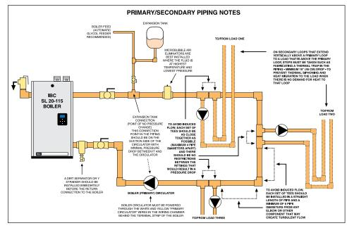
Figure 25: Important Primary/Secondary piping details with closely-spaced tees
